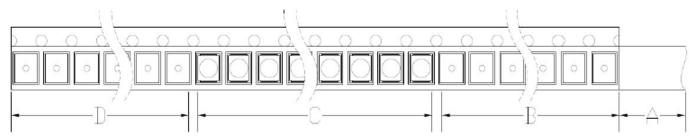
A: Top Cover Tape, 300mm; B: Leader, Empty, 200mm; C: 2000 Lamps Loaded; D: Trailer, Empty, 200mm.
