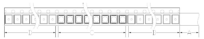
A: Top Cover Tape, 300mm; B: Leader, Empty, 200mm; C: 2000 Lamps Loaded; D: Trailer, Empty, 200mm.
